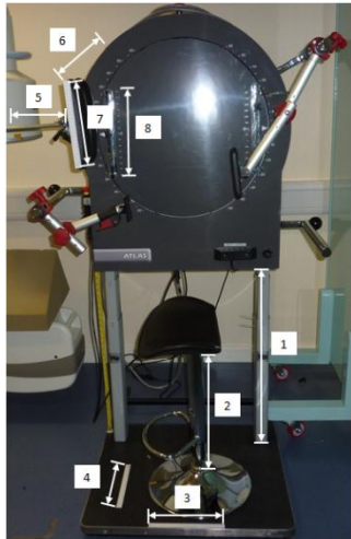
Figure 1: Stabilisation and motion-frame with aspects that were measured indicated (1-8)
